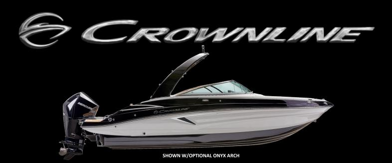
OVERALL LENGTH WITH ENGINES: 26' 10" LOA W/OUT ENGINE: 24' 6" BEAM: 102" MAX DRY WEIGHT: 5120 LBS DEADRISE: 19° FUEL: 53 GAL MAX HP: 300
