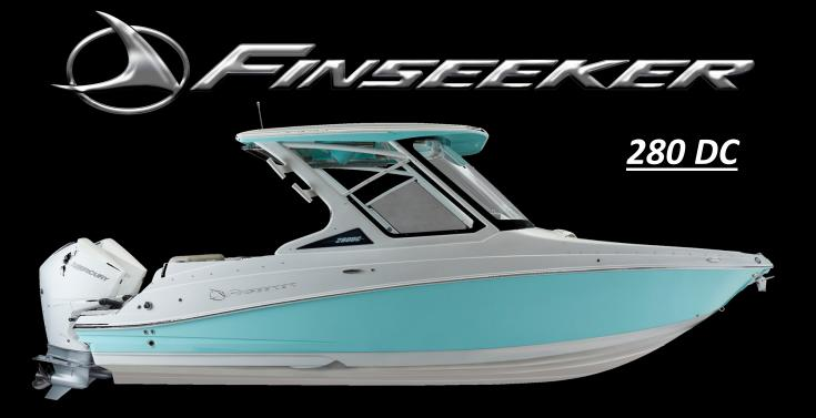
**OVERALL LENGTH W/ENGINES: 29'** LOA W/OUT ENGINES: 26' 10" **BEAM: 112"** MAX DRY WEIGHT: 8900 LBS **DEADRISE: 22°** FUEL: 165 GAL **BAITWELL: 26 GAL MAX HP: 600**
