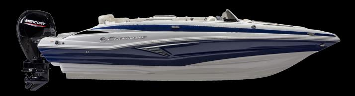
OVERALL LENGTH W/ENGINES: 22' 7" LOA: 20' 4" BEAM: 102" MAX DRY WEIGHT: 3725 LBS **DEADRISE: 19°** FUEL: 45 GAL **MAX HP: 200**
