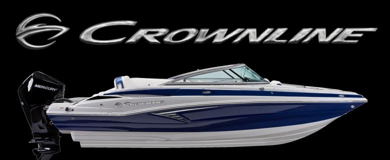
**OVERALL LENGTH W/ENGINES: 23' 9"** LOA: 21' 4" **BEAM: 102"** MAX DRY WEIGHT: 4060 LBS **DEADRISE: 19°** FUEL: 45 GAL **MAX HP: 250**
