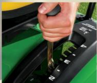
**Cutting Height Adjuster.** Cutting height can be adjusted in 1/4 in. increments for a precise, even cut. (Shown here on the D100 Series.)
