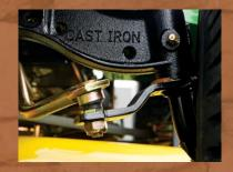
**Front axle** is constructed of solid cast iron for extra durability.
