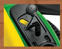
D105 Lawn Tractor features an **Automatic Transmission**. Just like your car, you simply set your direction with the fender-mounted hand control and press your pedal to select your speed.
