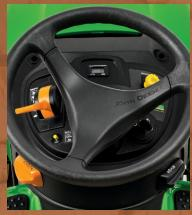
**Electric PTO**, available on some models, provides instant engagement of mower blades. Ignition switch and single lever throttle/choke are on the dash within easy reach.
