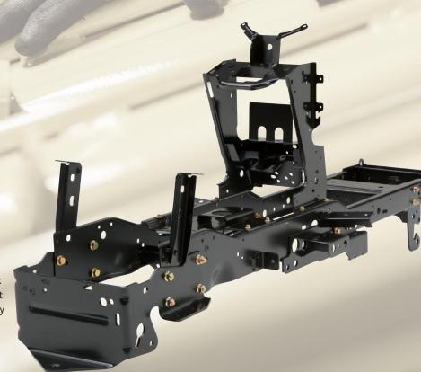
A heavy-duty robotically welded frame. The bedrock of these machines. So solid, it can handle an amazing variety of heavy-duty attachments.
