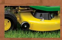
The mower decks are stamped out of high grade steel with a rounded design to leave no corner or edge for grass to get stuck in. This helps the cut grass to travel easily through the deck and supports an even dispersal for a quality cut.
