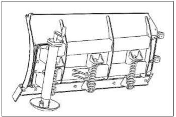
**Installation steps:** Fasten the support adjustment component to the left main shovel with M12\*30 bolts (D15) according to the position in the above figure.
