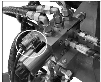
The solenoid valve head harness is fastened to the solenoid valve by inserting the phillips screws on the solenoid valve
