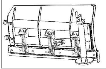
**Installation steps:** Fasten the support adjustment component to the right main shovel with M12\*30 bolts (D15) according to the position in the above figure.
