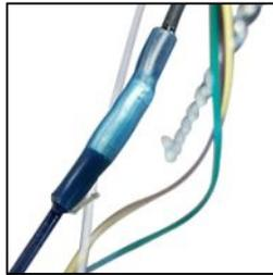
**Heat-Shrunk Sealed, Concealed Wiring**
